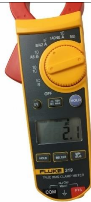
Figure 7. Measuring full load current after adaptation to 3phase 380 grinding machine
