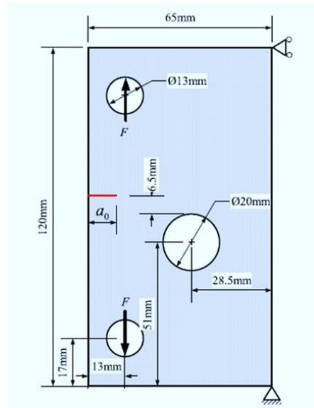
Figure 8. Geometric dimensions of the second problem.
