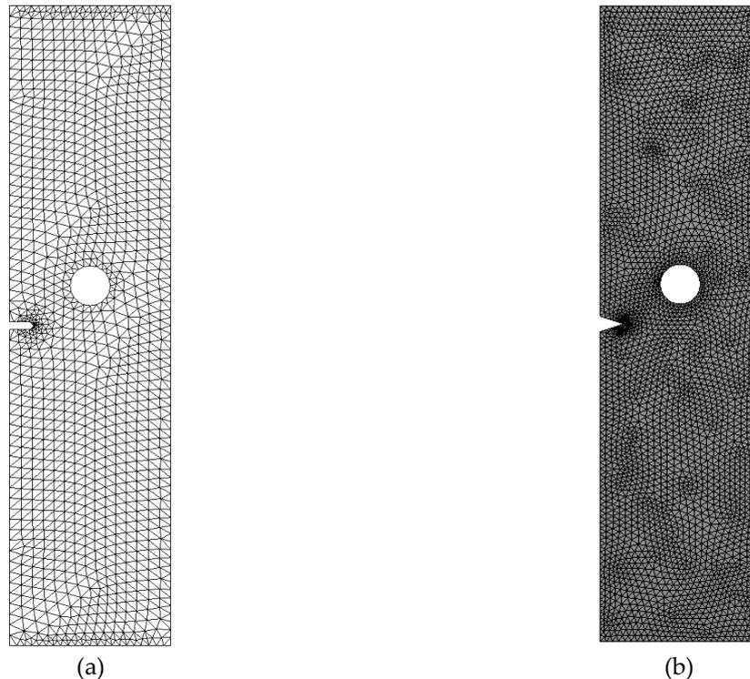
Figure 4. Initial mesh: a) Franc2D/L, b) ANSYS.
