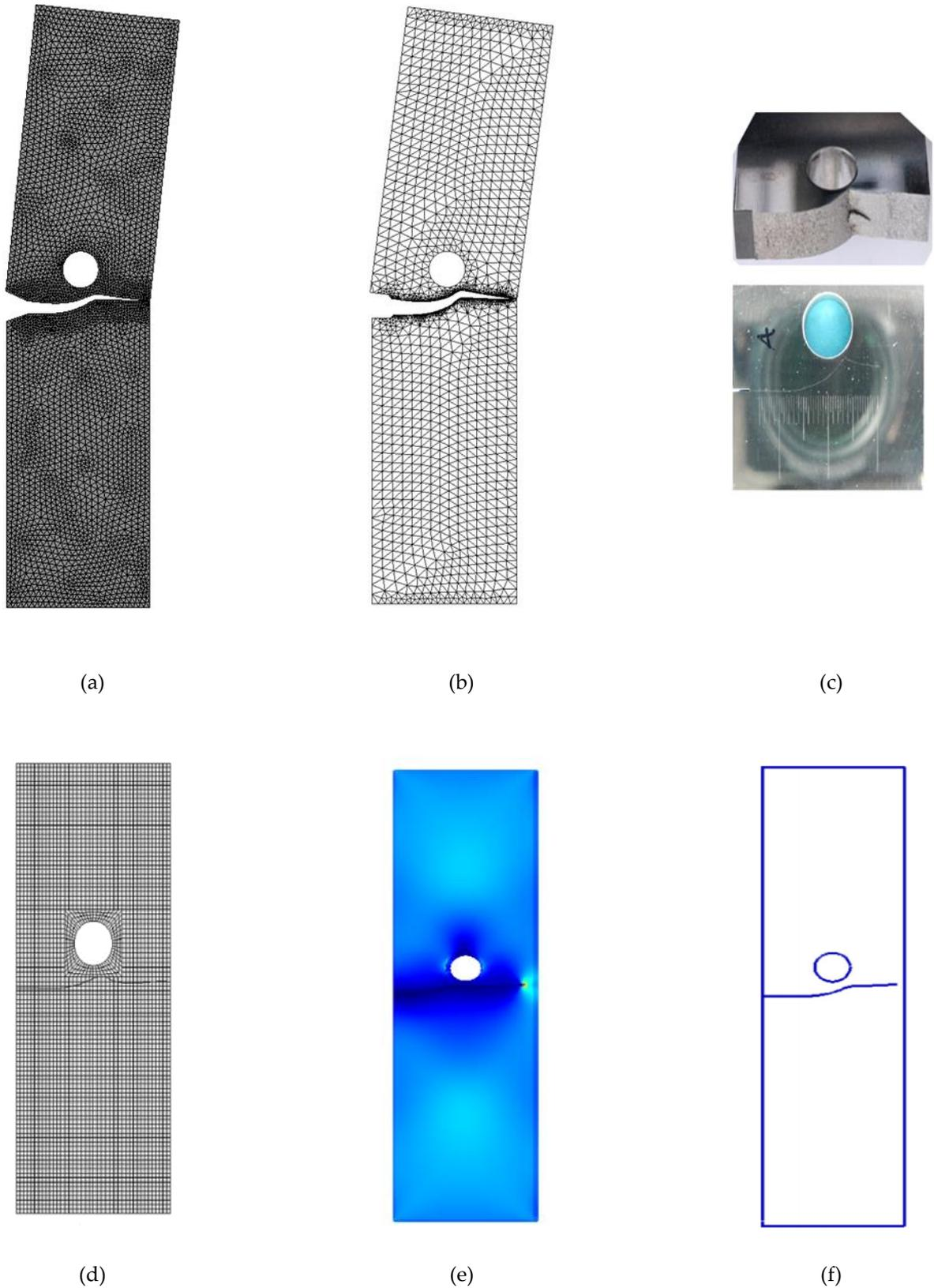
Figure 5. Comparison of crack growth trajectory (a) ANSYS, (b) Franc2D/L, (c) Experimental (Varfolomeev et al.(Varfolomeev, Burdack et al. 2014)), (d) Numerical (Varfolomeev et al.(Varfolomeev, Burdack et al. 2014)), (e) Numerical (Wiragunarsa et al.'s (Wiragunarsa, Zuhail et al. 2021)) and (f) Numerical (Liu et al. (Liu, Li et al. 2017)).
