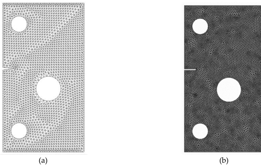
Figure 9. Generated Mesh: a) FRANC2D/L, (b) ANSYS.
