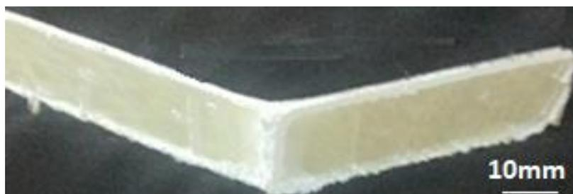
Figure 9. The mode of failure by impact of chopped-GFRP
