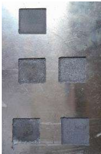
Figure 8. St. steel at different current 5, 10, 15, 20 and 25 Amp.
