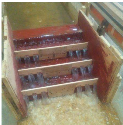
Figure 2. End sills provided with opening area at each side ( n=6 , with rectangular opening shape).
